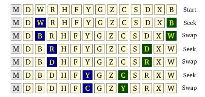
In the figure above, the pivot is M, the first letter in the list. The figure is broken down into "seek" phases, where we advance i and j, and "swap" phases, where we exchange the values at those indices. The blue highlighted letter on the left corresponds to the position of i and the green highlighted letter on the right corresponds to the position of j. Notice at the last step how they cross paths.
