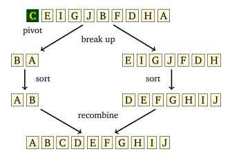
Notice that the way quicksort breaks up the array is more complicated than the way mergesort does, but then quicksort has an easier time putting things back together than mergesort does. Here is one way to implement quicksort, coded to return a new list instead of modifying the caller's list.
