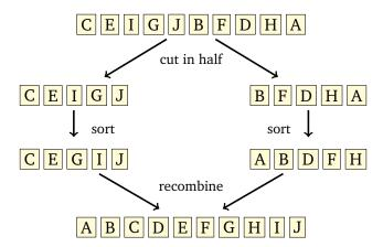
The way the merging process works is we have position markers (counters) for each of the two halves, each initially at the starts of their corresponding halves. We compare the values at the markers, choose the smaller of the two, and advance the corresponding marker. We repeat the process until we reach the end of one of the halves. After that, we append any remaining items from the other half to the end. The first few steps are shown below:
